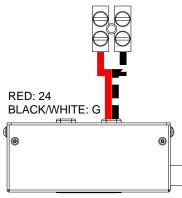
Use the included 3-position terminal block to connect the line input wires to the line power as shown in the following diagram.
